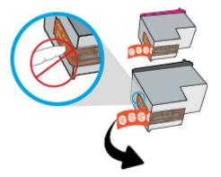
**5.** Insert the new cartridge, and then close the latch as illustrated.
