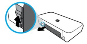
5. Insert the battery into the battery slot.
