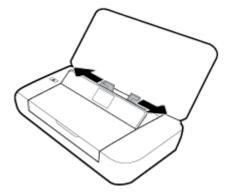
**3.** Insert the paper print-side up and slide the paper-width guides till they fit snugly against the sides of the paper.
