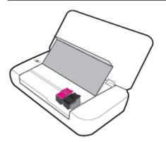
**CAUTION:** Do not replace or install cartridges when the print carriage is still moving.
